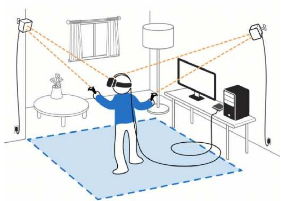
“Lighthouse” tracking system used in HTC Vive
